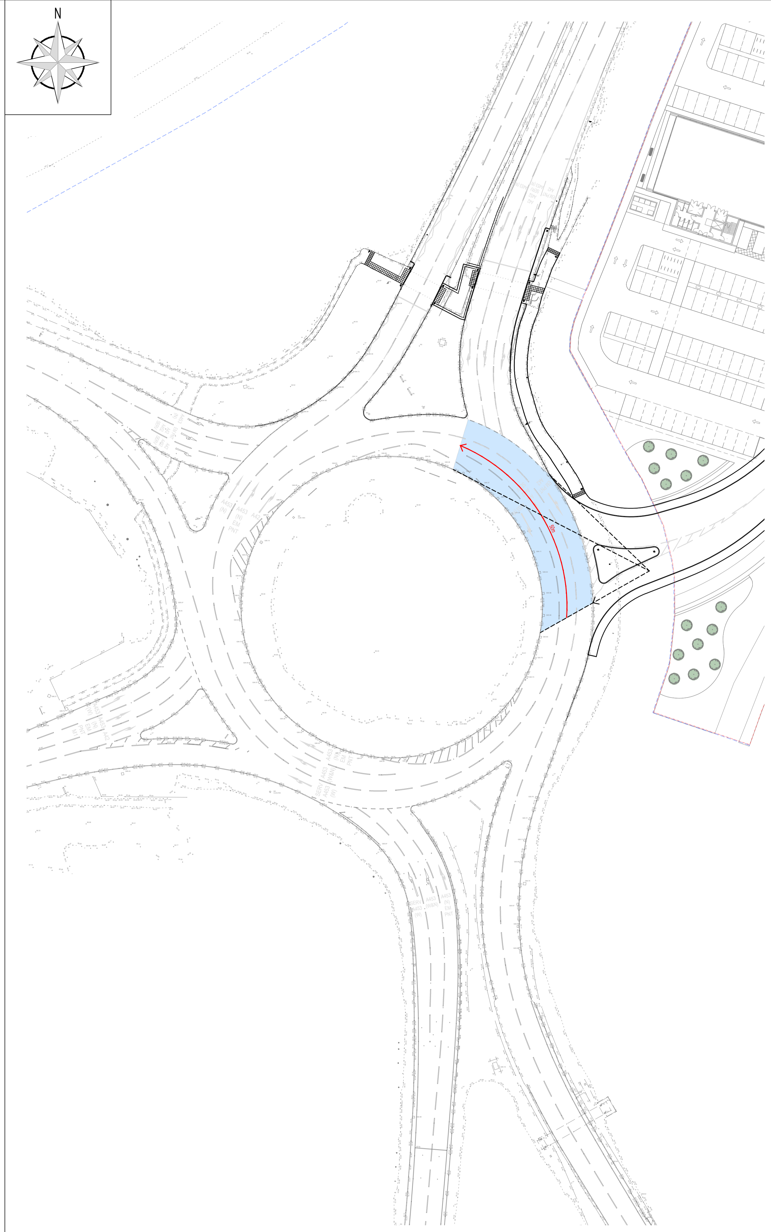
50m VISIBILITY SPLAY MEASURED TO THE RIGHT ALONG CIRCULATORY CARRIAGEWAY 15m IN ADVANCE OF GIVEWAY LINE
